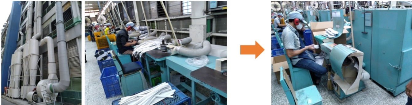
Figure 2.4.9: Replace large exhaust fans with small exhaust fans
