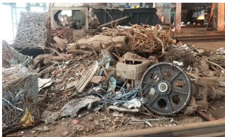
Figure 4.3. Scrap material is fed into the furnace in various sizes.
