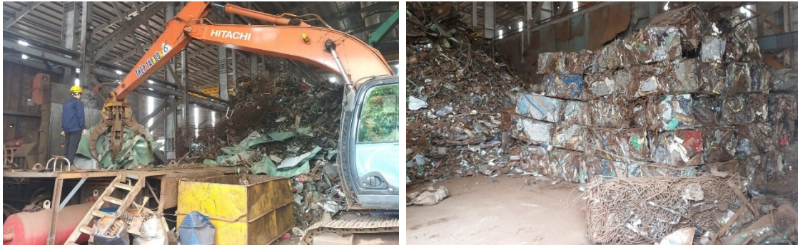
Figure 4.2. Hydraulic pressing machine and the scrap blocks after pressing.
