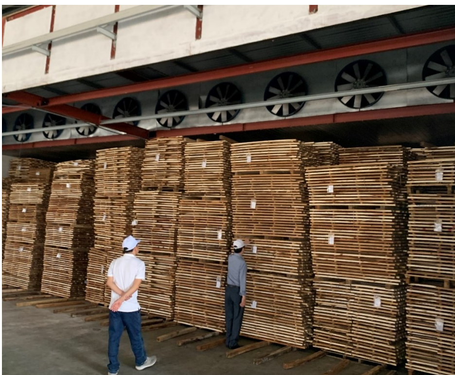
Figure 1 Typical example of a batch dryer in Vietnamese wood processing industry.
